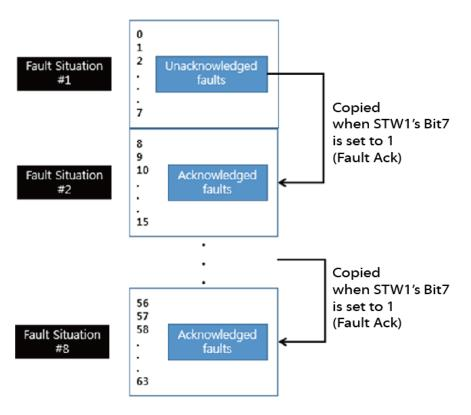
In the diagram, the current Fault Message is saved at Fault Situation #1. Each fault message is saved based on the time of occurrence, from index 0 to 63.
