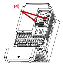
Mount PROFInet communication Module and fasten the removed screw(6) and the included screw(7).
